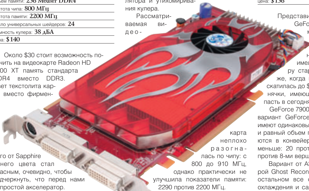
Sapphire Radeon HD 2600 XT 256 Mb GDDR4
