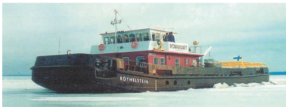
The shallow draught diesel-electric icebreaker Röthelstein, with Azipod propulsion
